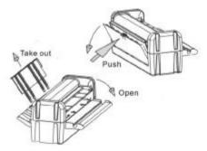
Open the front cover by pushing the latch and take out the sliding tray that is stored inside.
