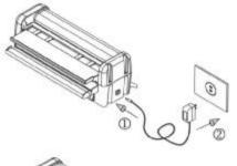
Connect the power lead to the socket on the side of the machine and then plug the adaptor/plug into an electrical outlet.
