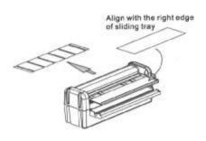
Now place a strip into the sliding tray. Align it to the right hand edge and push the tray forward gently with both hands until the machine takes up the drive. Each strip will be cut into five business cards. Repeat for the second strip.
